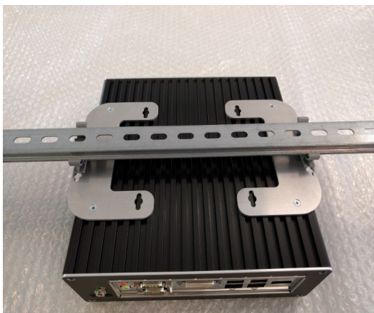
Fig. 2: Mounting on DIN rail(example)
