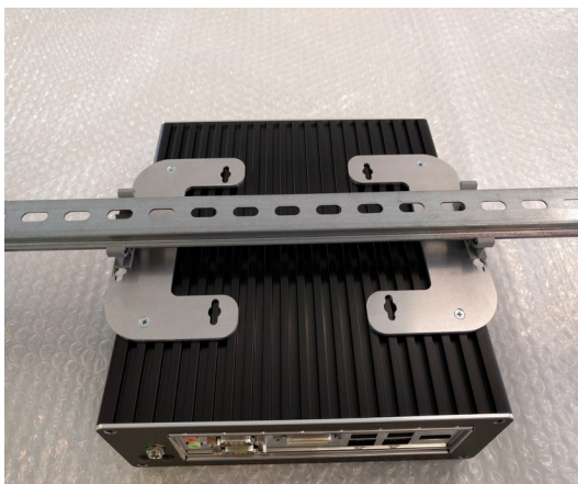
Fig. 2: Mounting on DIN rail(example)
